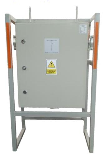
Switchgear type SPR1-AWX is an electrical device designed for use in the underground mining faces in non-explosive hazard conditions and on the ground in environment 2. Switchgear type SPR1-AWX is designed for connecting and branching-off mine 3-phase grid circuits with insulated star point on the transformer (IT system) for the grid rated voltage of 500V.
